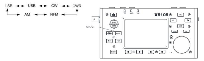
HOLD **[MODE]** to toggle between Split ON and Split OFF. In Split operation VFOA is used for receiving, VFOB is used for transmitting. When in Split operation, the split icon is visible beside the VFOB frequency.
