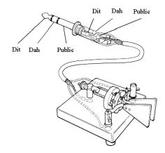
NOTE: The TRS jacks require a matching plug with a narrow shaft to allow complete insertion.
